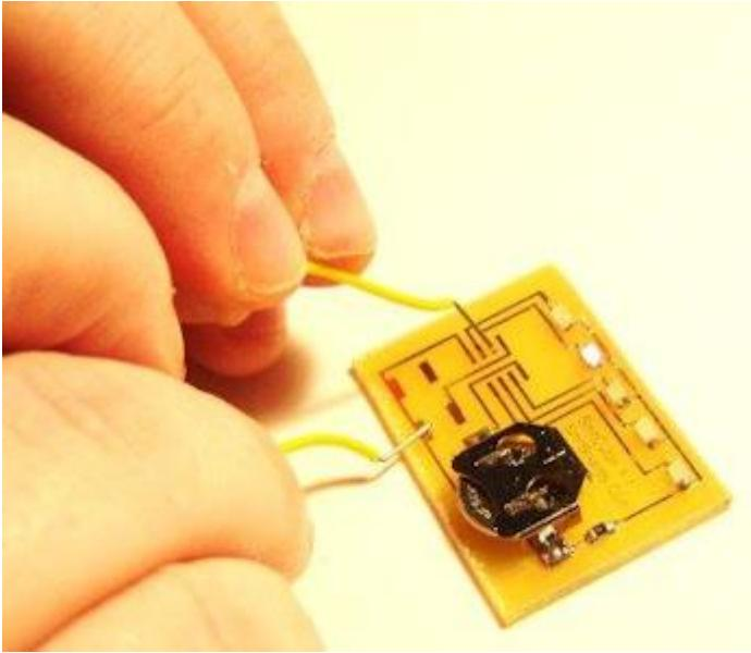
You may now test your work by temporarily inserting the battery, positive side up.
