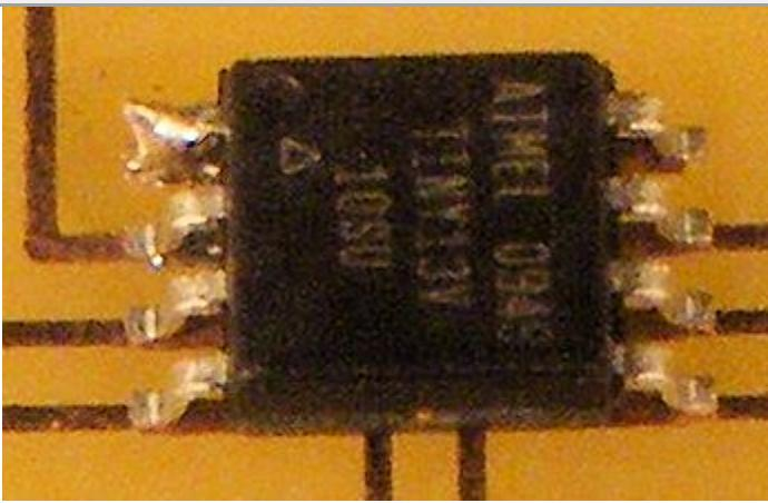
Here's a close up of the solder joint. Note that pin 8, just opposite pin 1 to the right, falls just short of its pad. You'll need to apply enough solder to make sure that pin 8 makes connection.
