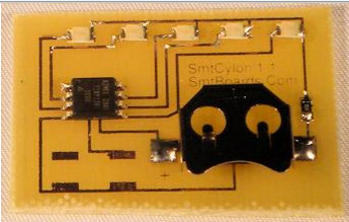
Next, probably the most difficult solder of the kit. Drop a dab of solder on the top left most pad for the CPU. Orientate the CPU with the small dimple to the upper left, That's pin 1. Push the CPU into the hot solder, Lining up the remaining feed on the correct pads.
