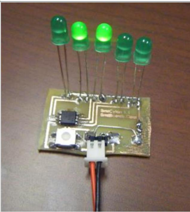
Nothing says that you have to assemble the kit exactly as shown. The SMTCyron can be used as a control circuit for full sized LEDs powered by a 5v power supply. I have a spare mutant version 1.1 to torture, so I tied the positives together, something I corrected in 1.3, and soldered in a power connector. Works pretty well...
