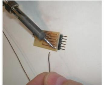
Begin by soldering the right angle connector from the back of the board.
